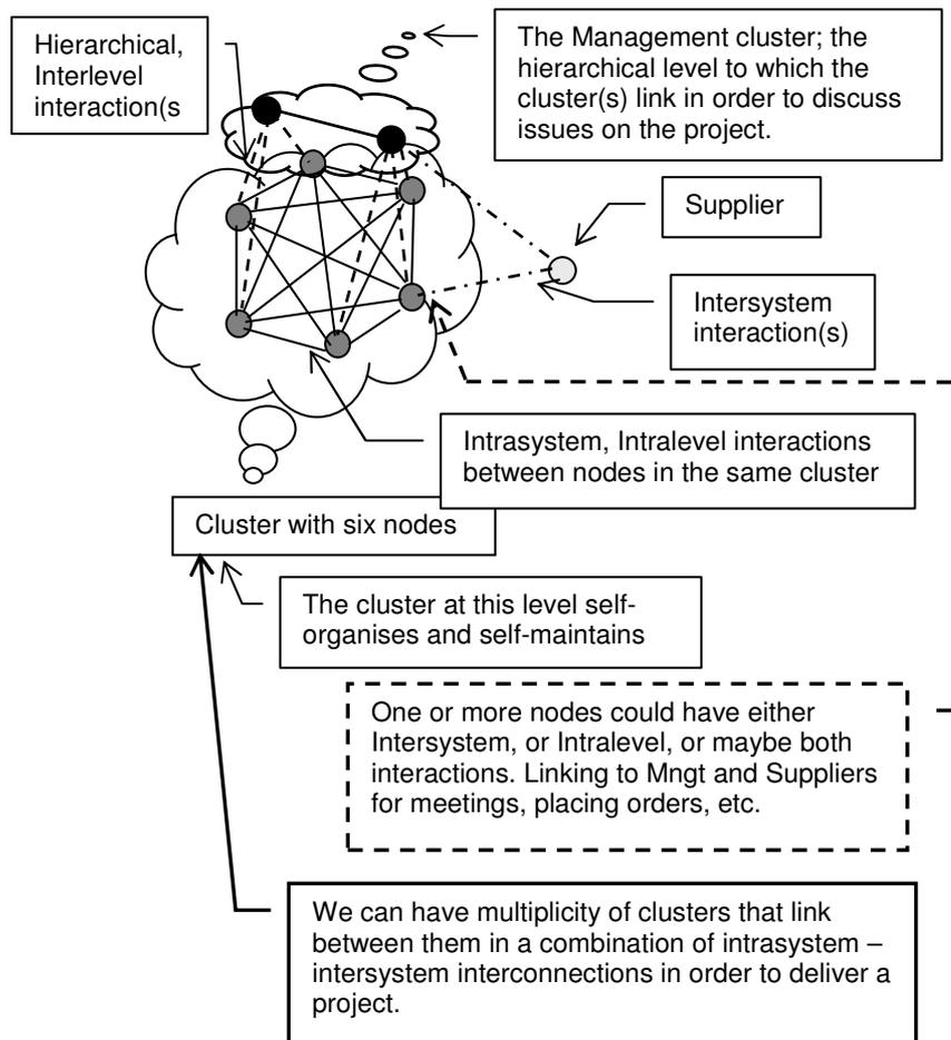
Figure. 10.5 depiction of interconnections between construction clusters at various levels.
